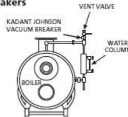
Typical application of a Kadant Johnson Vacuum Breaker as used on a steam boiler to break a vacuum imposed when a boiler is shut down, thereby condensing the steam in the boiler and creating a vacuum. This condition causes the boiler to be flooded by pulling in excess water from the return system.
