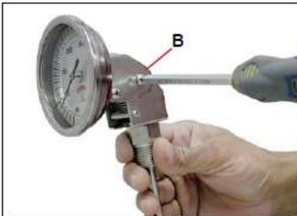
To tilt thermometer head up to a 90° angle or straighten it, loosen single screw (B) by 1/2 turn only.
