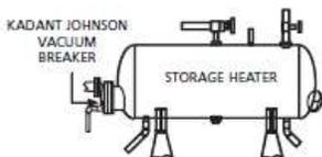
Horizontal storage heater with heating coils protected by a Kadant Johnson Vacuum Breaker.
