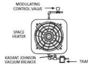
Typical space heater installation with Kadant Johnson Vacuum Breaker protection.
