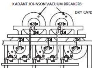
Textile dry cans, multiple slasher cylinders, print cans, etc., can be protected against collapse with Kadant Johnson Vacuum Breakers.
