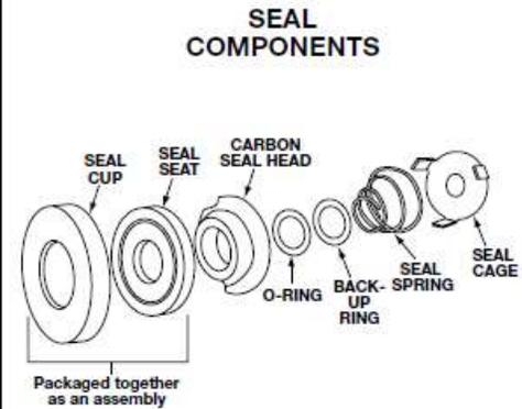
**INSTRUCTIONS FOR REPAIRING MECHANICAL SEAL**
