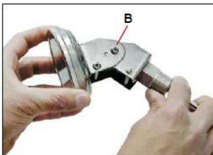
Tilt to desired angle or straighten. Retighten screw (B).
