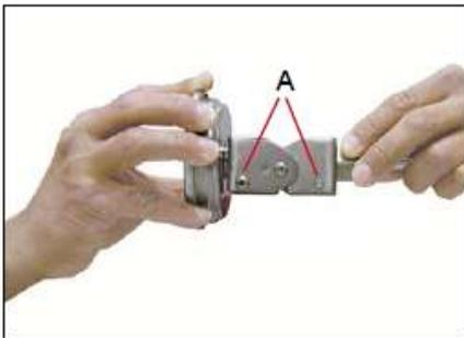
Now hold thermometer head and adjustable harness and rotate head to desired position. Retighten screws (A).
