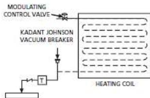
Kadant Johnson Vacuum Breaker installed on heating coil. When the modulating control valve closes, the steam in the coil will condense. A vacuum may exist in the coil even with the control valve partly open and positive pressure between the control valve and the coil.
