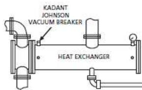
Typical installation of a Kadant Johnson Vacuum Breaker in a heat exchanger.
