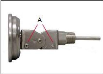
To rotate thermometer head up to 360°, make certain thermometer is in back connected position. Loosen two screws on both sides (A) until harness revolves freely.
