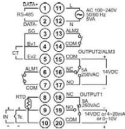
Wiring for 4 to 20 mA Transmitter Inputs
