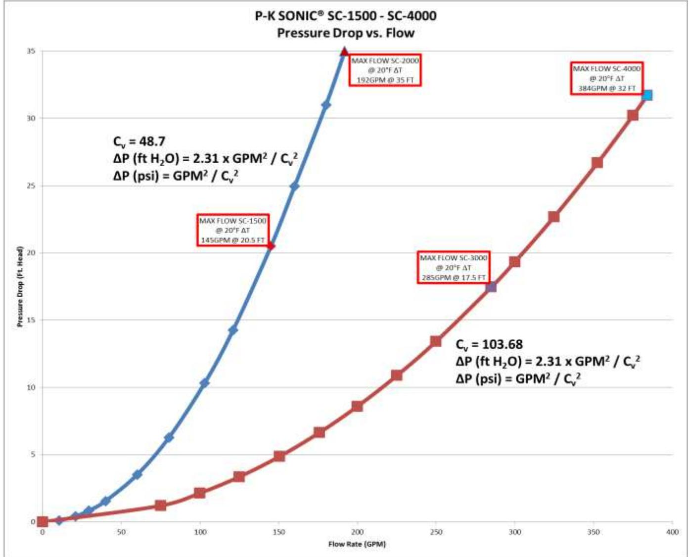
P-K SONIC® SC-1500 through SC-4000 Boilers: Minimum & Maximum Flow Rates
