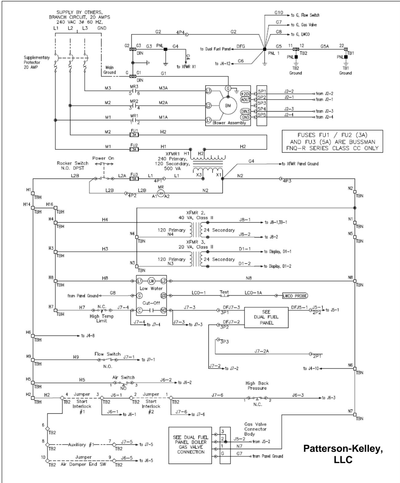
IF ANY OF THE ORIGINAL WIRE SUPPLIED WITH THIS BOILER MUST BE REPLACED, IT MUST BE REPLACED WITH THE SAME UL WIRE TYPE.
