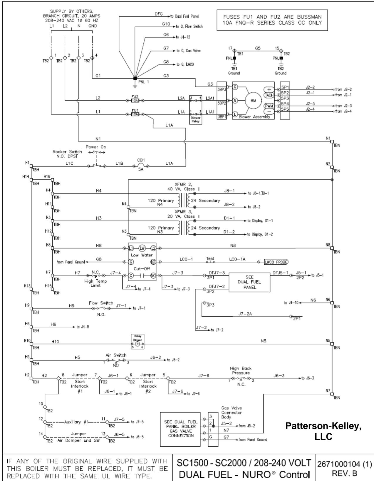
IF ANY OF THE ORIGINAL WIRE SUPPLIED WITH THIS BOILER MUST BE REPLACED, IT MUST BE REPLACED WITH THE SAME UL WIRE TYPE.
