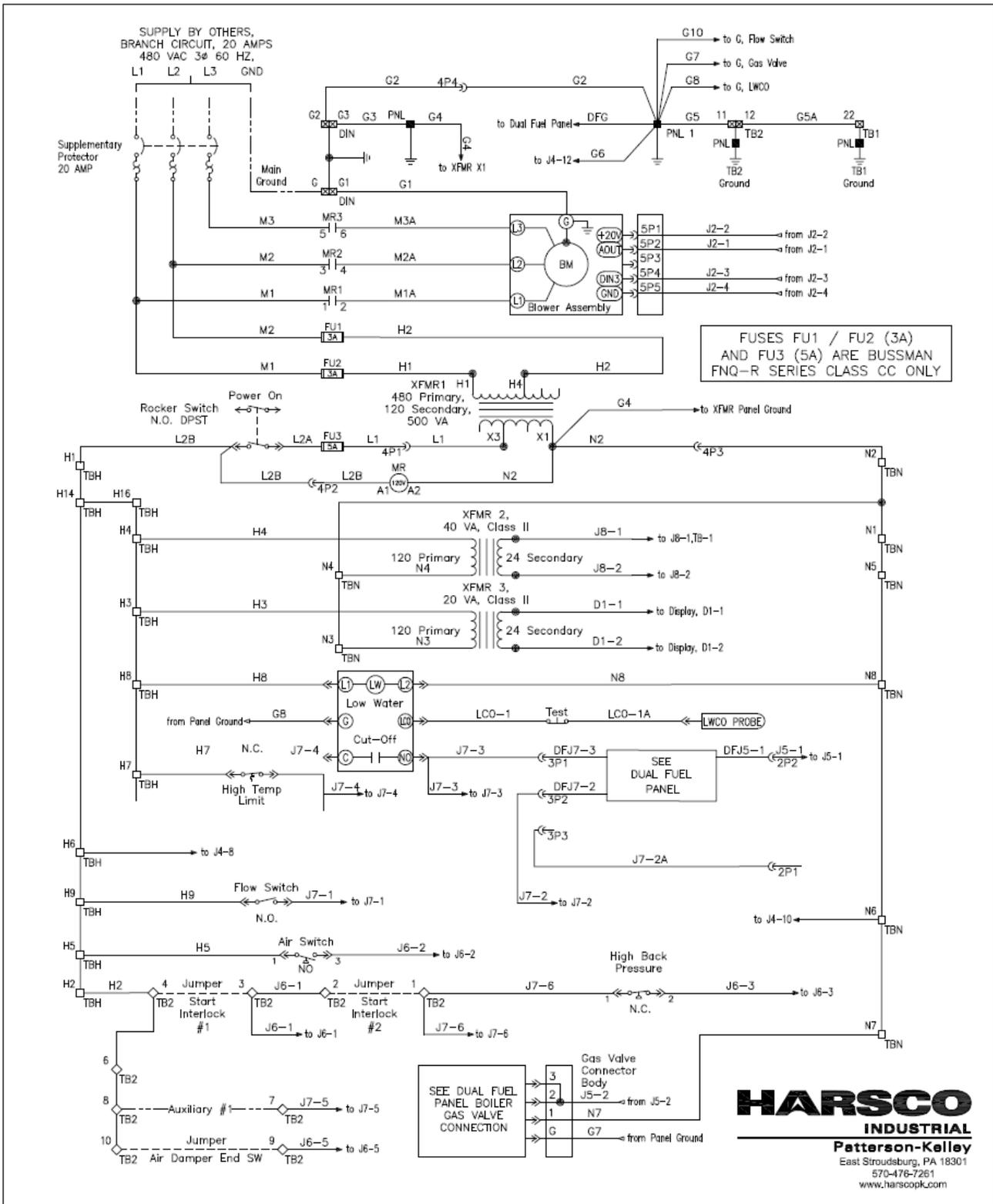
SI LES CÂBLES D'ORIGINE FOURNIS AVEC CETTE CHAUDIÈRE DOIVENT ÊTRE REMPLACÉS, ILS DOIVENT ÊTRE REMPLACÉS PAR UN CÂBLE DE MÊME HOMOLOGATION UL.
