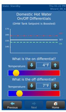
For Pool Heater models, program the NURO as Domestic Hot Water being the pool water values.
