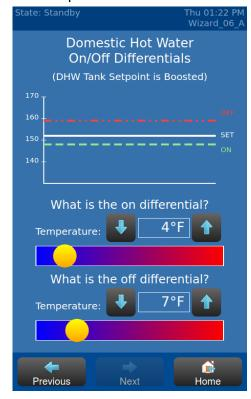
Once the "on differential" and "off differential" are programmed, press **<NEXT>** to proceed. The NURO will present a confirmation screen with a 30 second countdown timer. Press **<HOME>** to return to the home screen, or simply wait for the timer to expire. The MACH 'n' Roll  $^{\text{TM}}$  system is now programmed to respond to the aquastat installed in the domestic water storage tank.
