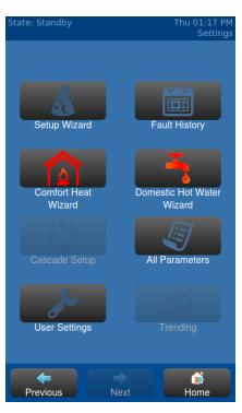
The next step of the Setup Wizard explains the Relay Instructions. The NURO® control system features four configurable relay outputs labeled RELAY A through RELAY D. The factory-default settings are recommended for most installations, but customization is possible. For more information on the configurable relay outputs, please refer to the NURO Boiler Controller: Advanced User's Guide, Part Number is 1004905979. Press **<NEXT>** to proceed.
