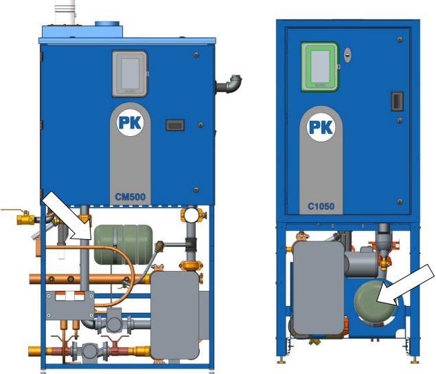
Use a pressure gauge to verify the air pressure is at least 12 psig. If the pressure is insufficient, use an air pump with built-in pressure gauge to charge the air pressure to a **minimum of 12 psig** before making ANY mechanical connections. The maximum air pressure need not exceed 20 psig.
