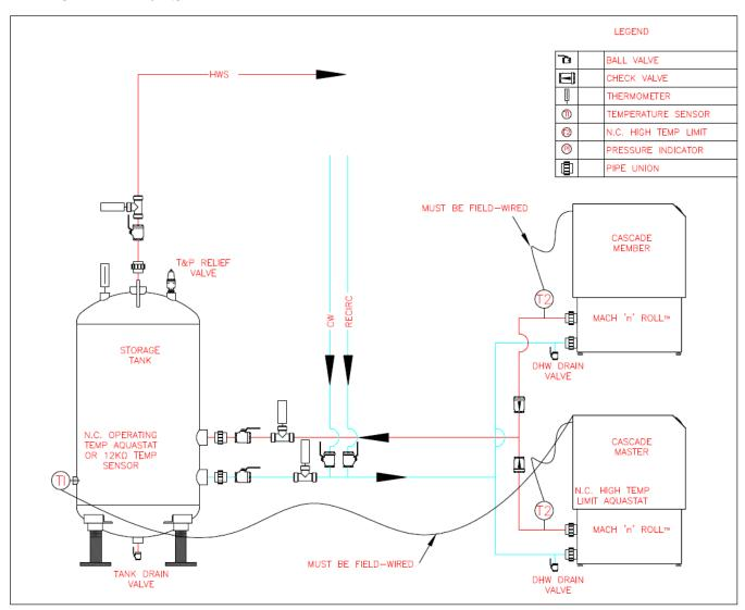
**NOTE:** Ensure a check valve is installed on the DHW supply piping of each MACH 'n' Roll<sup> $^{\text{M}}$ </sup> in the system. This will ensure the hot water is directed to the storage tank, and isn't allowed to backflow through offline MACH 'n' Roll<sup> $^{\text{M}}$ </sup> units.
