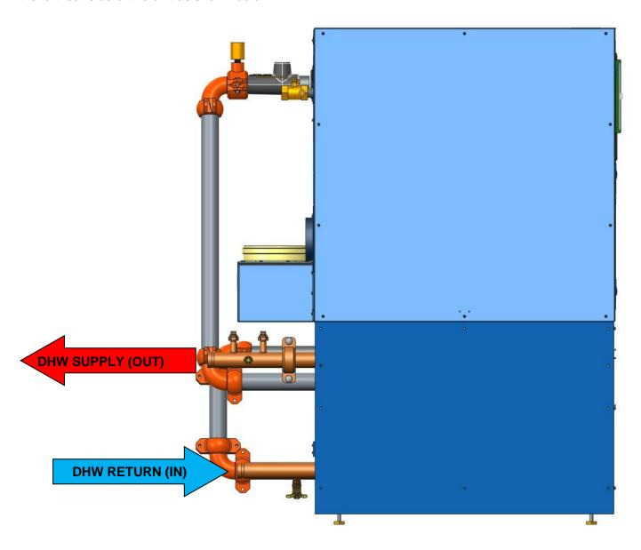
**NOTICE!** There are a variety of ways to connect to the domestic water piping on the MACH 'n' Roll™, but any sweat/soldered connections **must** use lead-free solder. Also, any brass or bronze pipe fittings, isolation valves, unions, check valves, etc. must also be lead-free.
