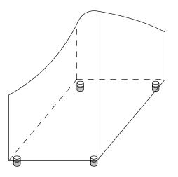
Adjustable Legs for Leveling and Floor Clearance
