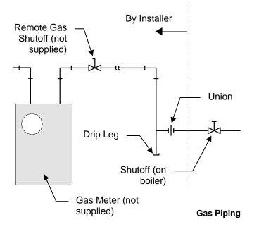
**Note:** Install a sediment trap (drip leg) and a union connection ahead of the primary manual shutoff valve
