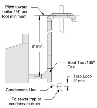
The first turn from horizontal to vertical should be made with a 135° boot tee. A tee cover with a condensate drain shall be provided at the bottom of the boot
