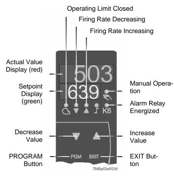
The diagram shows the RWF40 after switching on power. This condition is called the basic display. The actual value and the currently active setpoint are shown here. Manual operation, self-setting, and the user, parameter, and configuration levels can be activated from here.
