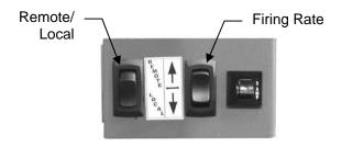
**Remote/Local and Firing Rate Switches**
