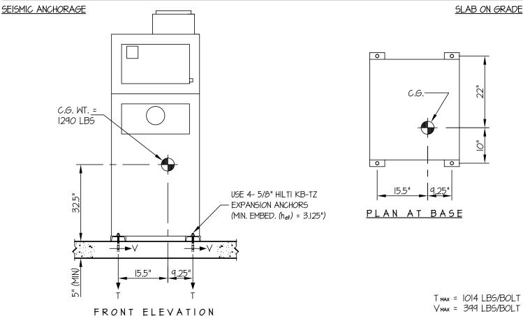
LOADS: PER 2010 CALIFORNIA BUILDING CODE SECTION 1613A AND ASCE 7-05 SECTIONS 12 AND 13. WEIGHT = 1290 LBS
