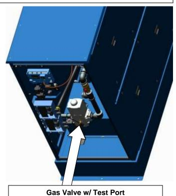
pressure on the gas train components. Each boiler is furnished with a manual shut-off valve which has an integrated test port. This port is located on the upstream side of the valve body for measuring supply pressure.
