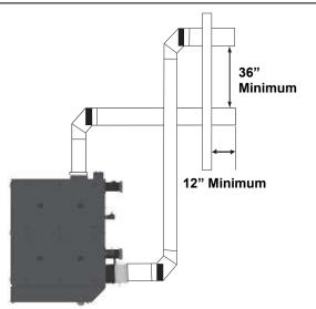
The combined pressure drop of the air supply duct and exhaust vent must not exceed 0.44" W.C. This pressure drop includes both the inlet and exhaust duct friction loss. If the air inlet and the exhaust vent terminate on the same wall of the building they must utilize the same type of termination fitting. Allowable termination fittings are either 90° elbows or tees. This boiler may be installed with sidewall vent using room air, see 3.4.1.
