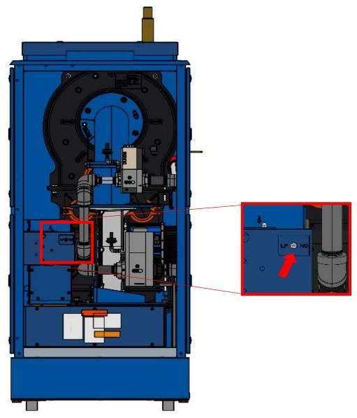
**A WARNING** If operating with Natural Gas, ensure the Propane Gas valve/cock is **CLOSED.** If operating with Propane Gas, ensure the Natural Gas valve/cock is CLOSED. Failure to do so could result in equipment damage, injury, and/or death.
