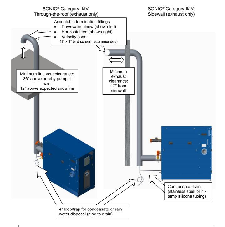
**Note:** For **Category II** installations, ensure the flue venting system is designed to maintain a slightly negative exhaust pressure between **-0.01**" **W.C. and -0.05**" **W.C.**
