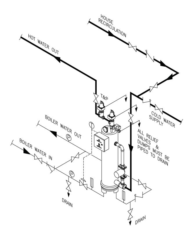
**Boiler Water 2 way piping**
