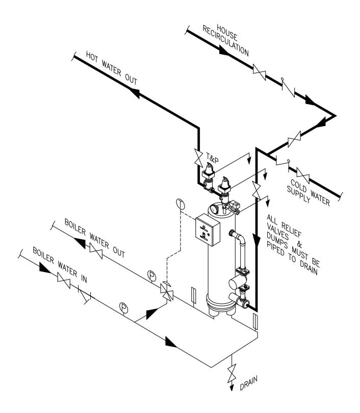
**Boiler Water 3 way Piping**
