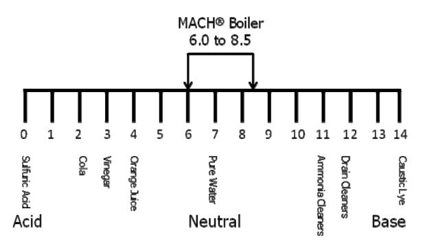
A sample of boiler water or boiler water/glycol should be tested. The sample should read between 6.0 and 8.5 to be correct for a MACH<sup>®</sup> boiler. Samples that read above or below the specification are outside of the allowable operating range and may cause damage to the boiler. It has been found that water with the pH greater than 8.5 can have negative effects on the aluminum and may cause premature boiler failure.
