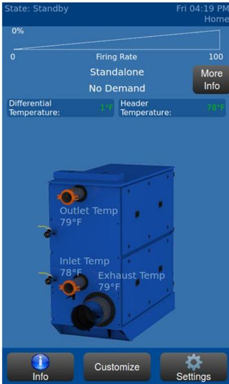
The NURO® control features a 7” color touchscreen display. The “Home Screen” (above) displays the general operating conditions of the MACH ‘n’ Roll™. To access additional temperature values and information, press <INFO> in the bottom left corner of the “Home Screen” which accesses the “Information” screen (right).
