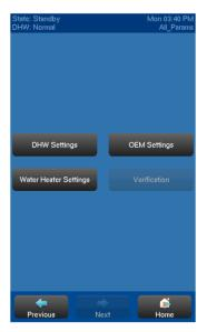
Shown right is **"All Parameters"** screen where **DHW Settings**, **OEM Settings**, and **Water Heater Settings** can be found.
