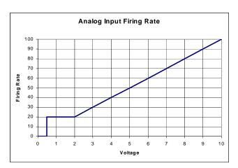
The control must be configured for analog input direct drive by setting parameter 34 to 02.
