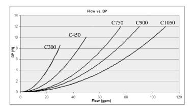
Proper flow rates may be achieved through a combination of primary and secondary flow loops. Multiple zones and pumps may result in different flow rates at different times. Consideration must be given to all possible conditions and their consequences.
