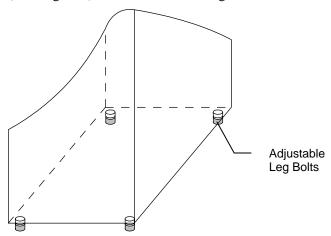
Adjustable Legs for Leveling and Floor Clearance
