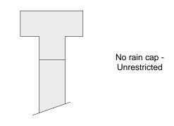
The roof intake termination must be an unrestrictive type, as shown above.
