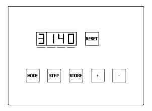
The MACH boiler is equipped with a combination combustion and temperature control. This control monitors combustion and lighting of the boiler, as well as maintaining temperature of the supply water. The temperature control portion modulates the boiler to maintain the desired outlet temperature based on the selected operating configuration.
