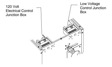
**Electrical Connections at Rear of Boiler**
