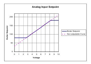
The control must be configured for a remote analog input setpoint according to the following table:
