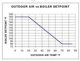
The control automatically detects the presence of the outdoor air sensor. If an outdoor air sensor is present, the boiler automatically defaults to outdoor air reset for setting boiler temp. The parameters should be set according to the following table:
