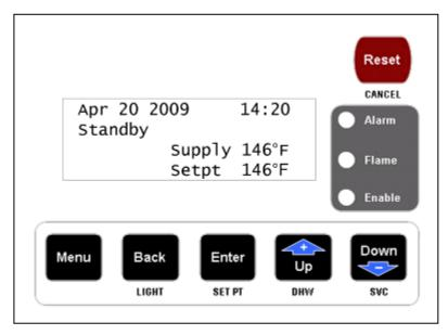
The P-K MACH boiler is equipped with the ENVI control; an intelligent control system with advanced features such as text-based display, communication capabilities, and boiler sequencing. Errors are date and time stamped providing built-in history of boiler status and performance. This control constantly tracks the load by recording burner high, low and mid run hours.
