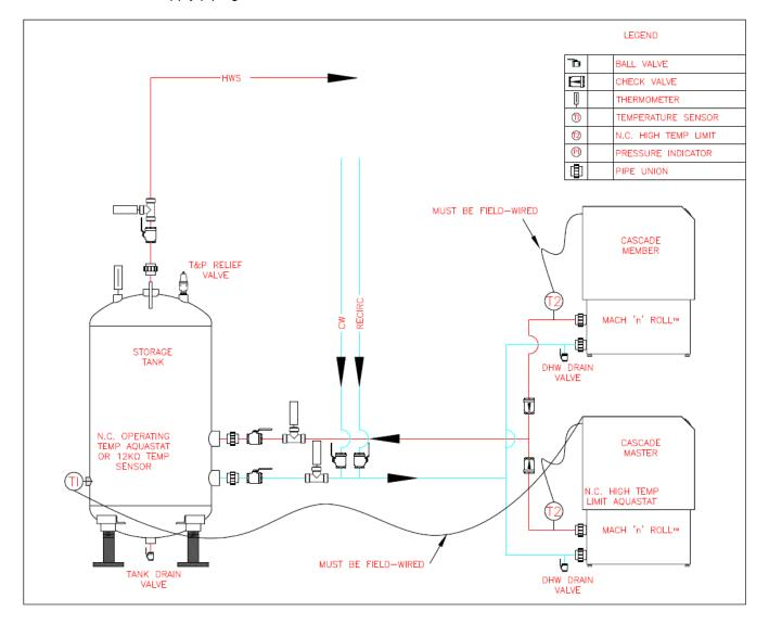
Ensure a check valve is installed on the DHW supply piping of each MACH 'n' Roll<sup>™</sup> in the cascade system. This will ensure the hot water is directed to the storage tank, and isn't allowed to backflow through offline MACH 'n' Roll<sup>™</sup> units. Refer to **Section 4.3** for setting up the ENVI controls for cascade operation. Also refer to **Sections 6.2 & 6.4** for detailed information on power wiring and controls wiring needed for cascade operation.
