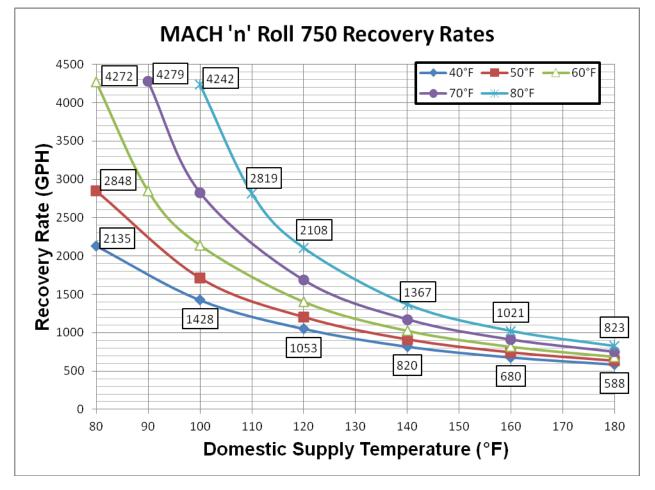
Choose the curve which most closely represents the incoming cold water temperature (40°F, 50°F, 60°F, 70°F, or 80°F). Move along the x-axis to the desired domestic hot water supply temperature. Move vertically until the intersection with the applicable curve. From this intersection, move horizontally to the left to determine the recovery rate of the MnR750 from the y-axis. Several sample recovery rate data points are included for reference.
