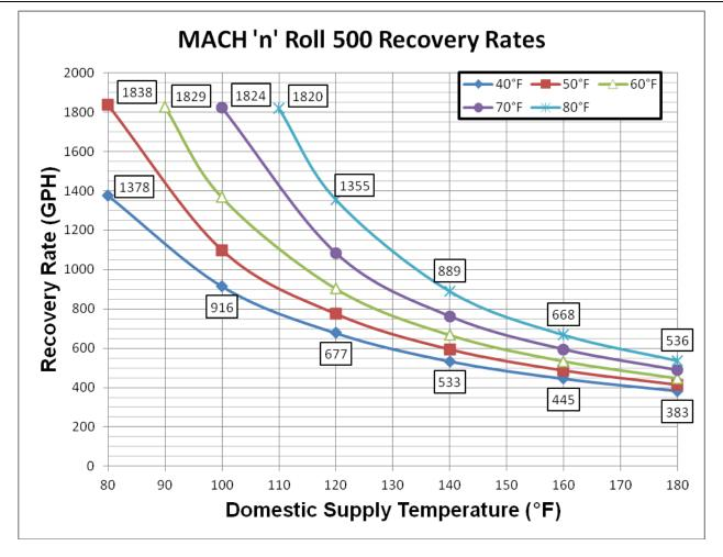
Choose the curve which most closely represents the incoming cold water temperature ( $40^{\circ}F$ ,  $50^{\circ}F$ ,  $60^{\circ}F$ ,  $70^{\circ}F$ , or  $80^{\circ}F$ ). Move along the x-axis to the desired domestic hot water supply temperature. Move vertically until the intersection with the applicable curve. From this intersection, move horizontally to the left to determine the recovery rate of the MnR750 from the y-axis. Several sample recovery rate data points are included for reference.
