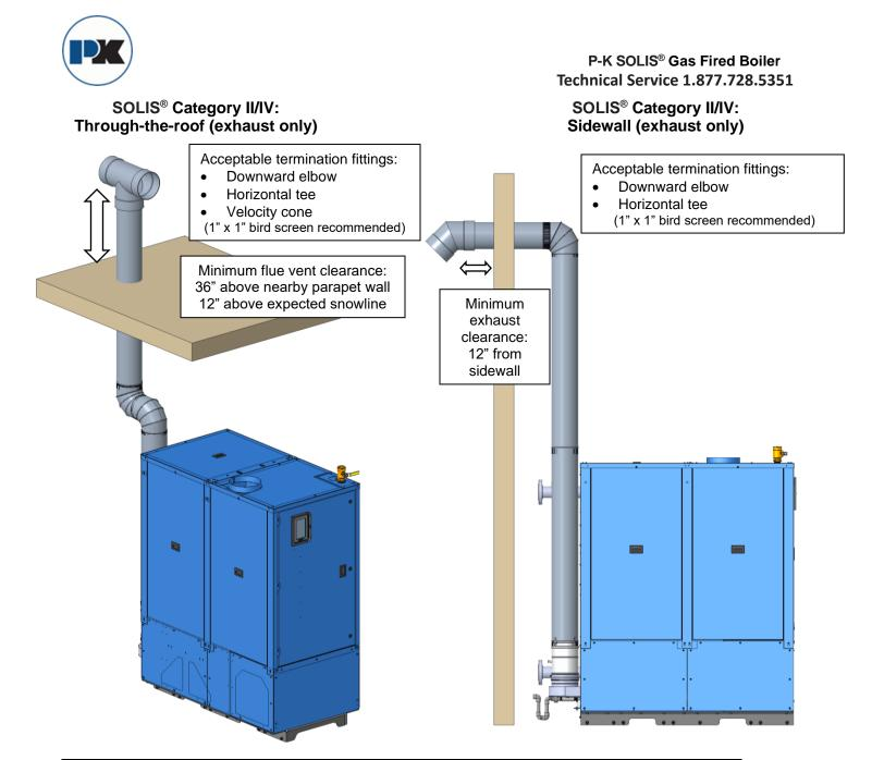
**NOTE:** For **Category II** installations, ensure the flue venting system is designed to maintain a slightly negative exhaust pressure **between -0.01**" **W.C. and -0.05**" **W.C.**
